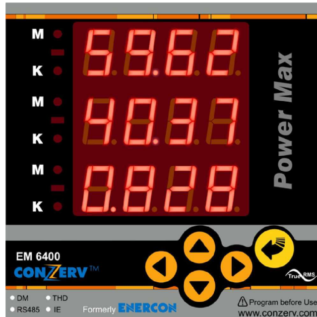
Figure 2.2: The Power Max EM 6400 front panel with display and keypad
